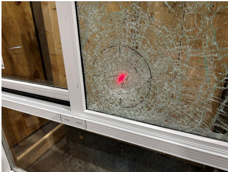
Photo No. 16 Specimen #4 – Impact #2
