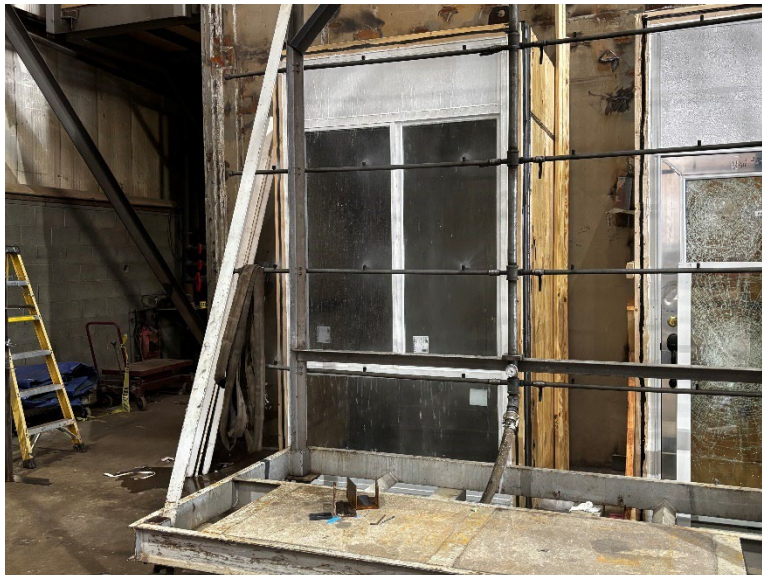
Photo No. 2 TAS 202 Static Water Penetration Testing
