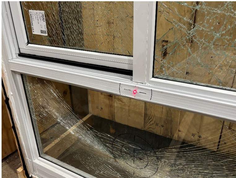
Photo No. 12 Specimen #3 – Impact #4
