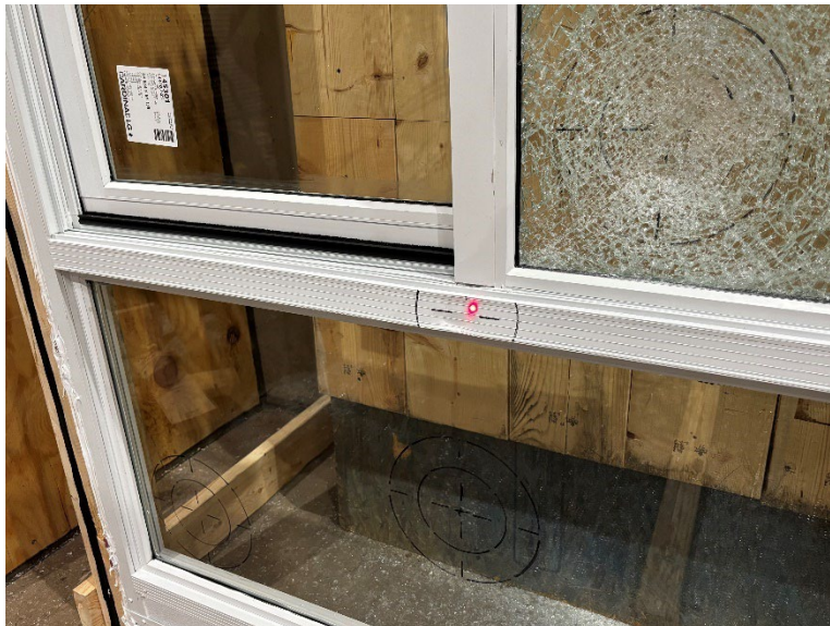
Photo No. 18 Specimen #4 – Impact #4
