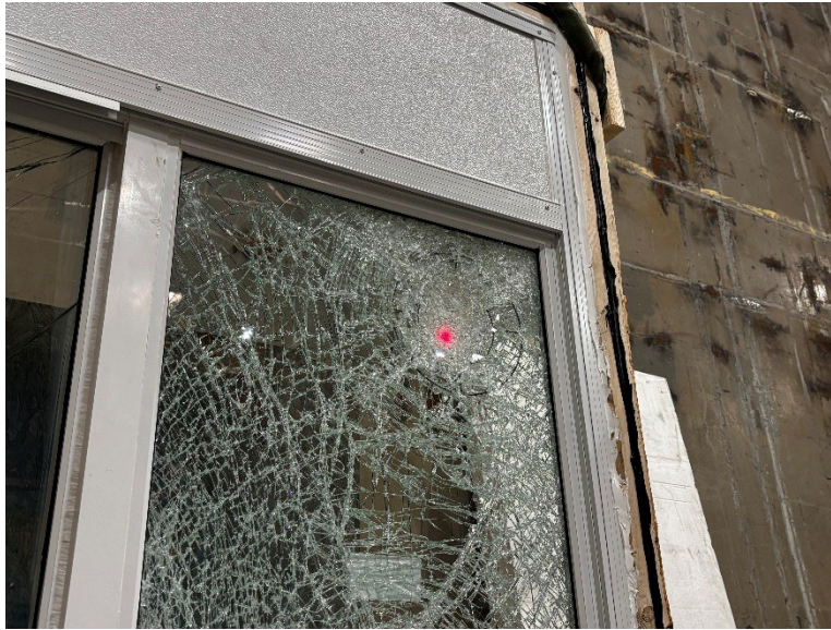
Photo No. 11 Specimen #3 – Impact #3
