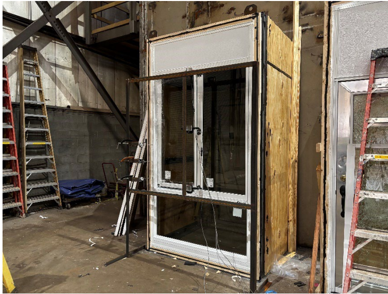
Photo No. 1 TAS 202/203 Indicator Setup
